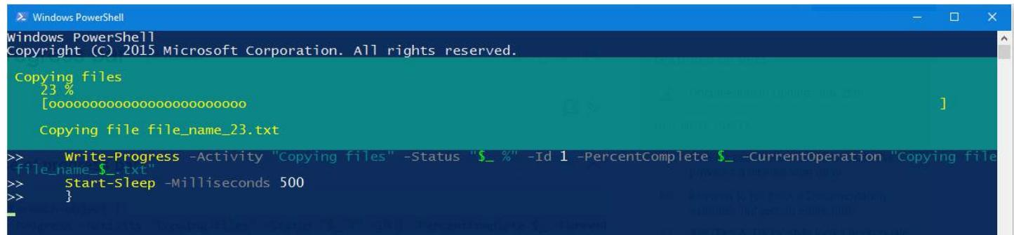
The screenshot shows a Windows PowerShell window. The command entered is a loop from 1 to 100 using `ForEach-Object`. Inside the loop, `Write-Progress` is used to display a progress bar for "Copying files". The status shows "23 %". The progress bar is filled with approximately 23 small blue segments. Below the progress bar, the message "Copying file file\_name\_23.txt" is displayed. The command `Start-Sleep -Milliseconds 500` is also visible at the bottom of the loop body.
